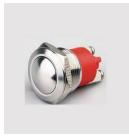
Diameter: Ø 19mm Switch Rating: 5A/250VAC Contact Configuration: 1NO Operation Type: Momentary The Front Shape: Ball The Crust Material:
