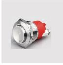
Diameter: Ø 19mm Switch Rating: 5A/250VAC Contact Configuration: 1NO Operation Type: Momentary The Front Shape: High The Crust Material:
